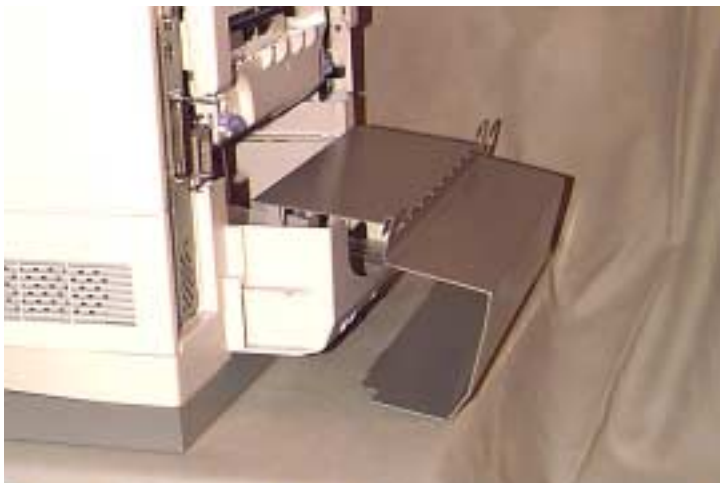
Access guard removed from rear allowing the lower paper tray to be withdrawn
