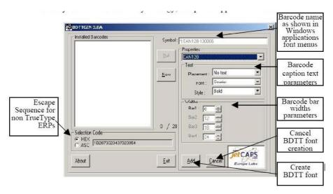
Note that the parameters available differ based on the symbology. For more information on the parameters, please refer to the BarDIMM 'Installation and Programmer's Guide, provided with the BarDIMM.
